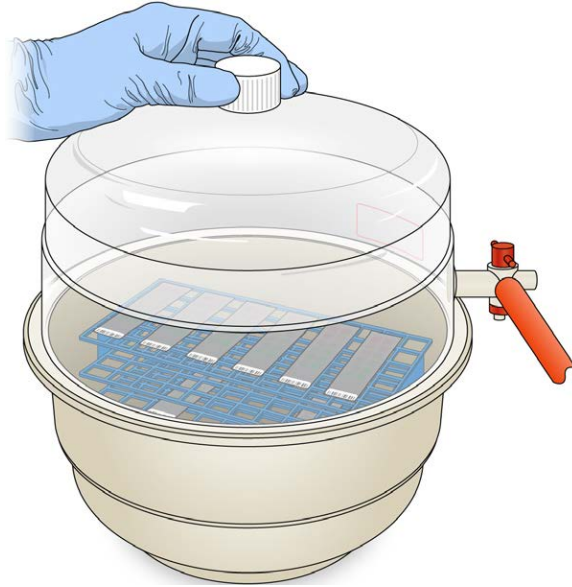
Figure 147 Testing Vacuum Seal
