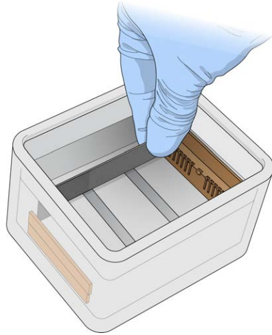
Figure 123 Submerging BeadChips in Wash Dish Containing PB1
