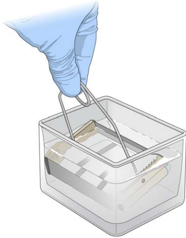
Figure 48 Wash Rack in Wash Dish Containing PB1
