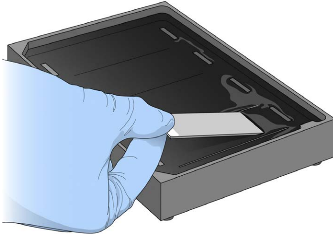
Figure 53 Placing BeadChip into Black Frame on Alignment Fixture
