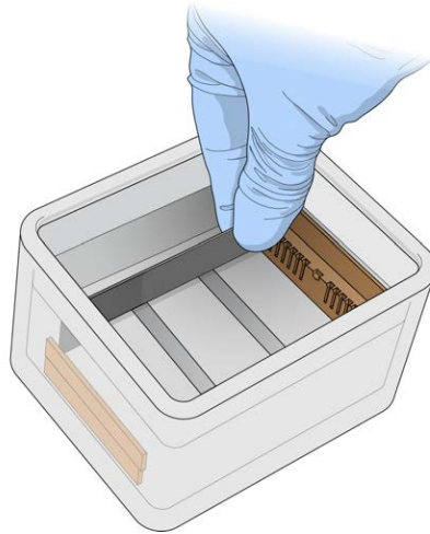
Figure 50 Submerging BeadChips in Wash Dish Containing PB1
