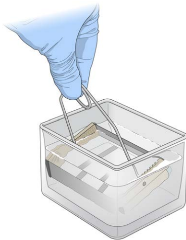
Figure 121 Wash Rack in Wash Dish Containing PB1
