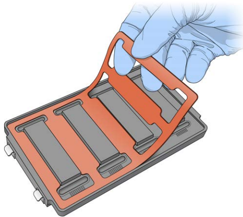
Figure 31 Placing Gasket into Hyb Chamber
