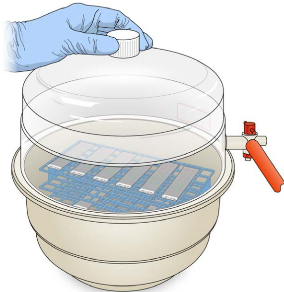
Figure 156 Testing Vacuum Seal
