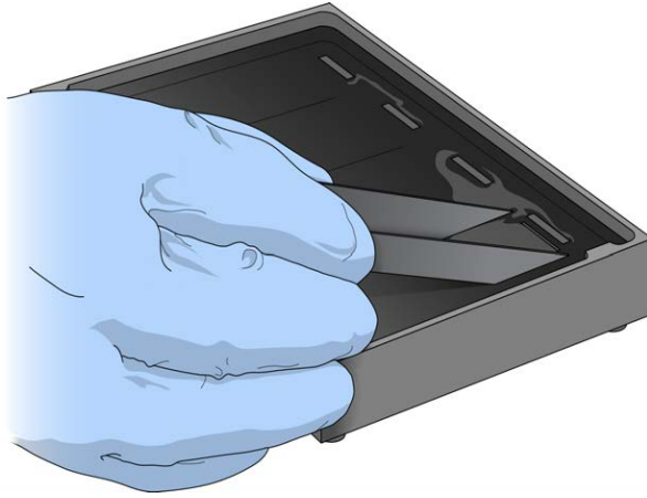
Figure 52 Placing Black Frames into BeadChip Alignment Fixture
