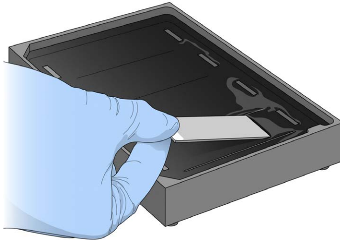
Figure 126 Placing BeadChip into Black Frame on Alignment Fixture
